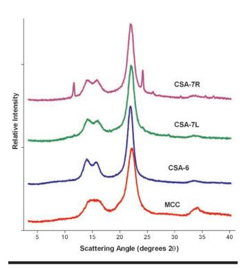
FIGURE 5. X-ray diffraction patterns of microcrystalline cellulose and the corresponding patterns obtained on the margins of the reference stamps Image used with the permission of *The Confederate Philatelist*.
