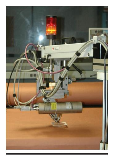
FIGURE 7. Bruker Artax XRF spectrometer.
