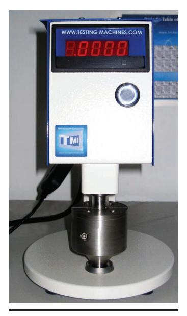
FIGURE 4. Testing Machines Inc. model 49-76-01 micrometer.
