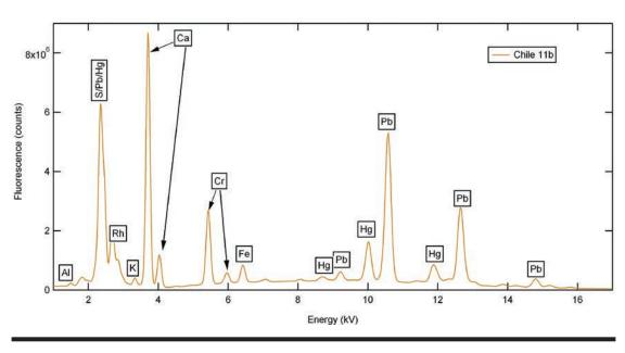
FIGURE 17. Sample of XRF results for Chile number 11.
