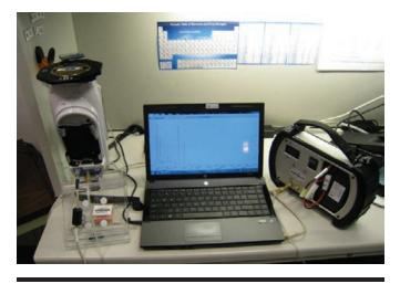
FIGURE 6. Bruker Tracer III-SD X-Ray Fluorescence Analyzer.
