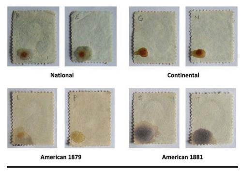
FIGURE 11. Iodine potassium iodide spot test for starch, indicated by a bluish-black stain. Only the 1881 issue tests positive. Test courtesy of Eric Greve, Hope College Department of Chemistry.
