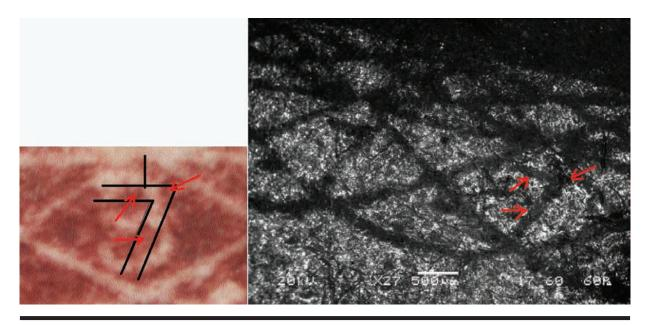
FIGURE 9. Right: Backscattered SEM image of stamp SK from the Victor Hugo cover. Note that all the uninked colorless areas appear dark on the image. Left: The red arrows indicate the area where the existing red ink must be altered/removed in order to produce a colorless figure "7" from the existing figure "3."
