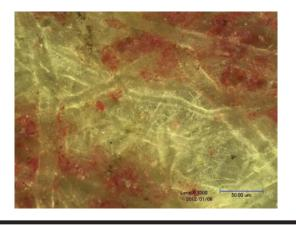
FIGURE 14. Depth composition analysis of the top of the right-hand "7" from stamp SL from the Victor Hugo cover. Such a recess of a colorless area can be produced only through impact between the plate and the paper at the time of printing and cannot be produced through faking.
