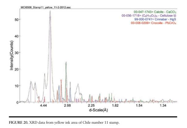
identification of the red spots in the yellow ink as vermilion (Figure 20). As in the FTIR, calcite was identified in all four inks. Crystalline fatty acid soaps were identified in the red ink. XRD of the paper areas of the stamps examined only identified cellulose of varying degrees of crystallinity.
