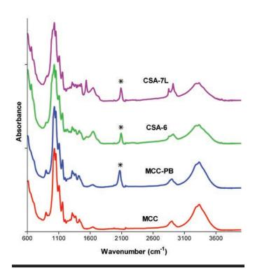
FIGURE 9. Infrared absorption spectra of microcrystalline cellulose, Prussian blue absorbed onto MCC, and the FTIR spectra obtained on the faces of the CSA-6 and CSA-7L reference stamps. The position of the Prussian blue peak has been marked, and it corresponds to feature I of Figure 8. Image used with the permission of *The Confederate Philatelist*.
