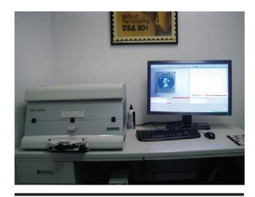
FIGURE 2. Video Spectral Comparator 6000 (VSC 6000).
