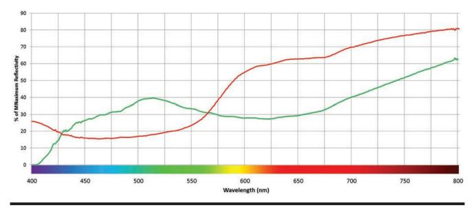
FIGURE 4. Reflectance curves from the VSC 6000 for typical red and green overprints.
