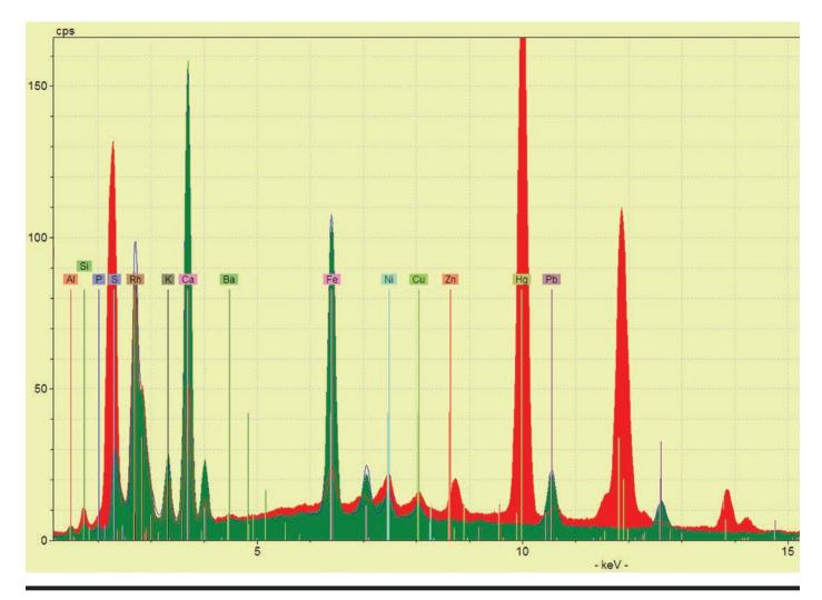
FIGURE 7. A typical spectrograph showing two different ink compositions (one in green, the other in red) based on simple elemental analysis using EDXRF. This allows the differences in ink composition to be easily discerned as the chemical elements are labeled.
