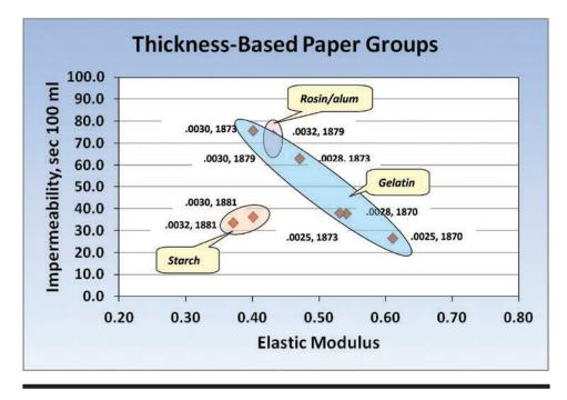
FIGURE 14. Mean elastic modulus versus mean permeability for each of the four thickness groups. Shaded areas enclose papers with the same sizing.
