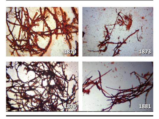
FIGURE 7. Cochineal red stain for distinguishing cotton from linen. Red indicates cotton; violet indicates linen. Staining and photomicrography courtesy of Robert Hisey.
