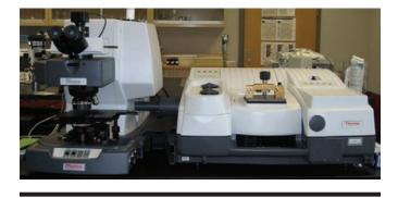
FIGURE 9. Thermo Nicolet FT-IR with Continuum microscope.
